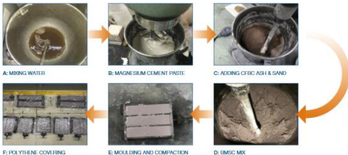
FIGURE 1: PREPARATION OF BASIC MAGNESIUM SULFATE CEMENT-BASED RPC
